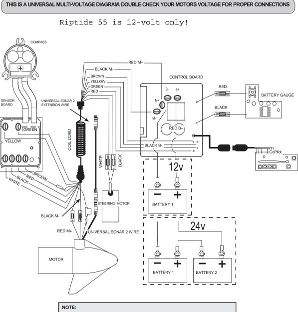
1. BATTERY 2 AND CONNECTING WIRE USED FOR 24V APPLICATIONS ONLY 2. UNIVERSAL SONAR 2 WIRES APPLICABLE TO US2 MOTORS ONLY
